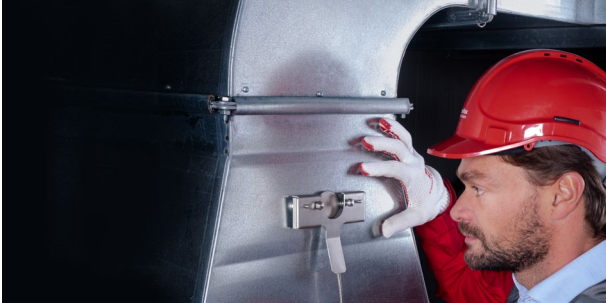
Figure 7 Mounting of IHF02 using an optional frame with magnets: note that optical properties of the sensor (black) do not match those of the metal object on which the sensor is mounted. This will lead to bad measurement data. (see also figure 3).
