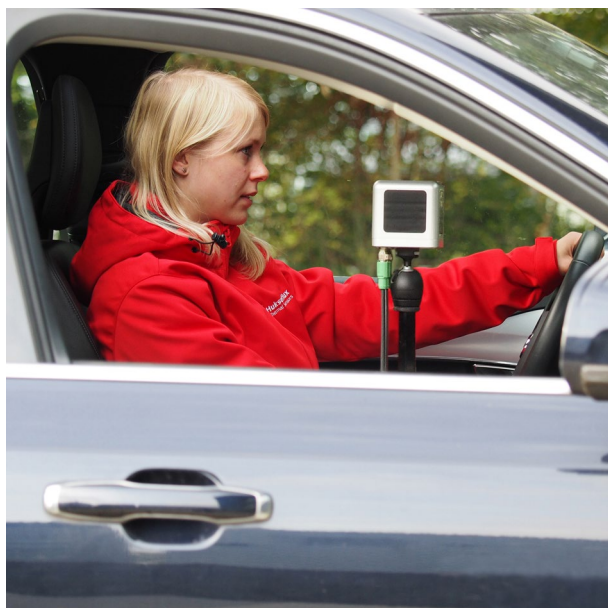
Figure 4 TCOM01 applied in car passenger comfort testing
