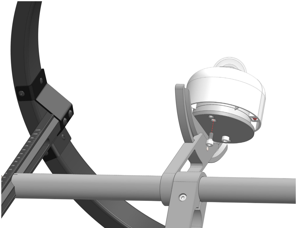
Figure 5.4.3.1.1 Mounting an SR15 pyranometer on SHR02
