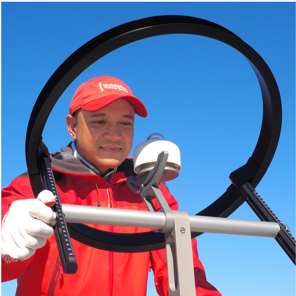
Figure 0.2 Installation of the SHR02 shadow ring with a Hukseflux pyranometer is easy.
