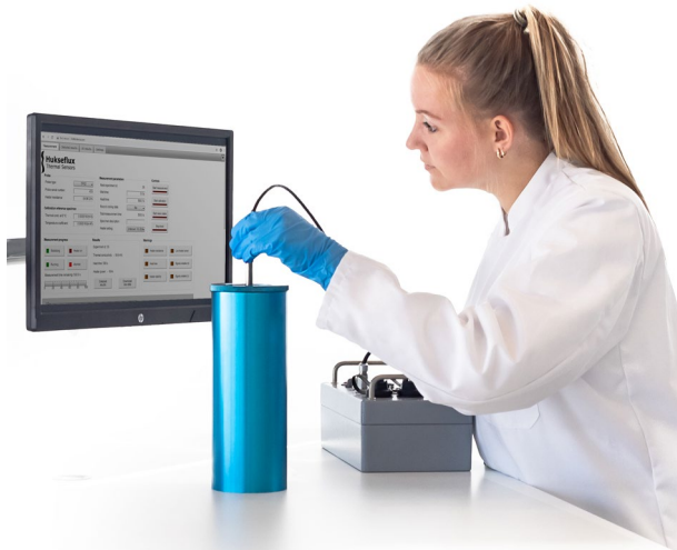
Figure 1 application of the complete TPSYS20 measuring system in a laboratory environment using a CRC01 calibration reference cylinder
