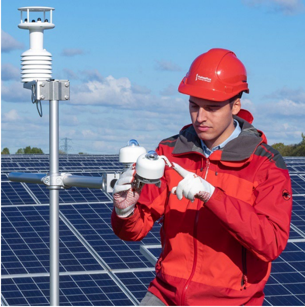
Figure 6 SR30 includes a digital tilt angle measurement, very practical for remote checks of instrument orientation. The image shows two SR30's in PV system monitoring, one measuring in Plane of Array (POA).
