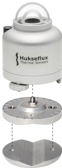
Figure 9 Optional spring-loaded levelling and tube mount for SR30. LM01 leveling mount (one part), TLM01 tube mounted (2 parts).
