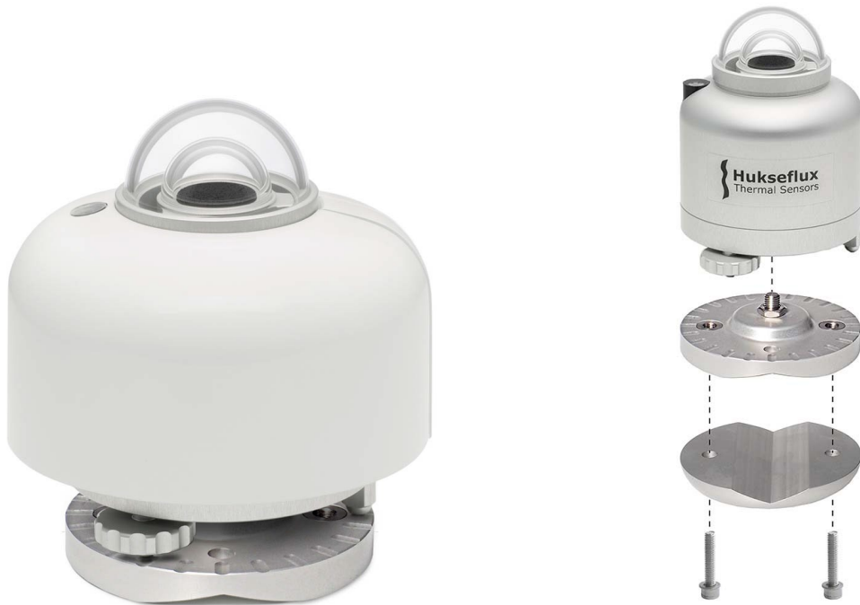
Figure 0.5 Optional levelling mount (picture on the left); a practical spring-loaded mount for easy mounting, levelling and instrument exchange on flat surfaces, and the optional TLM01 tube mount (picture on the right, two clamps) including spring-loaded levelling upper clamp (LM01 leveling mount, one clamp), plus a lower clamp for tube mounting and two sets of bolts.
