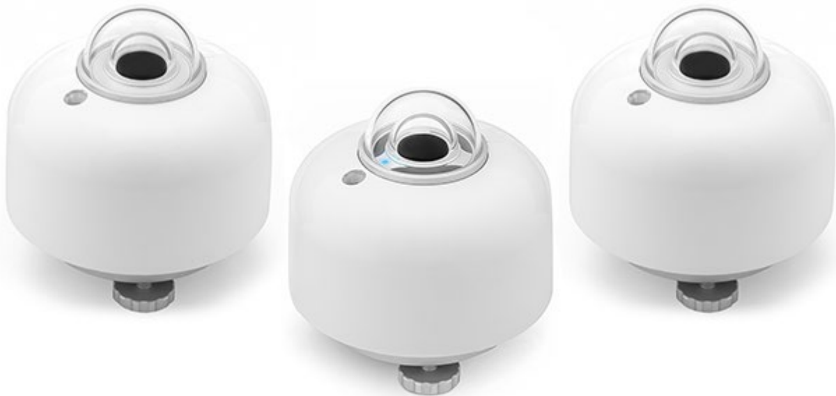
Figure 1 Industrial pyranometer models SR300-D1, SR200-D1 and SR100-D1. In front the leading Class A model SR300-D1, with heating, tilt sensor and the blue status LED. Left and right the non-heated Class A model SR200-D1 and Class B model SR100-D1.
