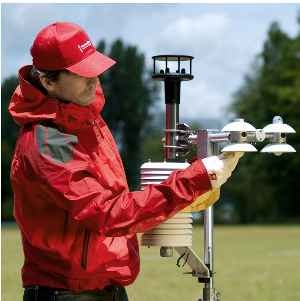
Figure 2 NR01 in use in a typical meteorological station.
