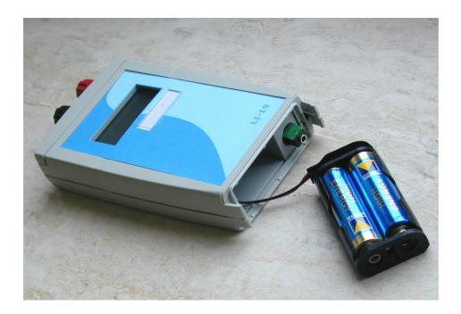
To prevent that the LI-19 is switched off while logging, the on/off switched is mounted so that the button has to be pressed quite deep to switch the LI-19 on or off. You can feel it and hear it when the switch toggles. Press the small black button far enough with your nail or a pencil until you feel and hear it switch.
