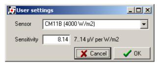
Use the wizard to select the sensor model that is to be used, and then enter the sensitivity of the sensor. The LI-19 is then ready to be programmed with the new settings. To do that, click the 'Program' button.
