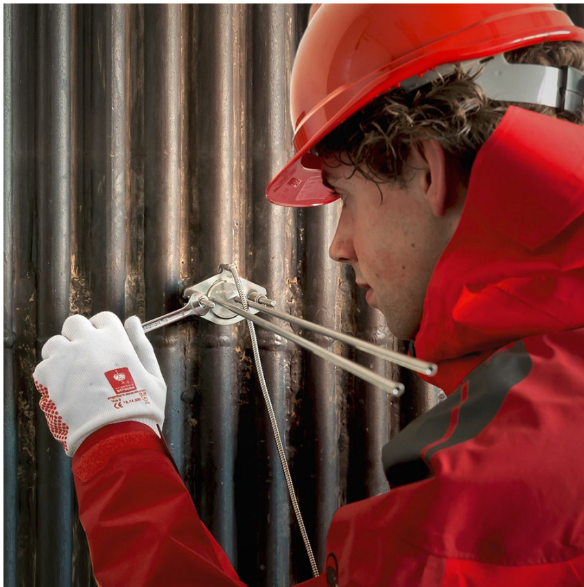
Figure 4.1.1 Example of an industrial heat flux sensor mounted on a boiler wall using tack-welded threads and spring-loaded bolts. The sensor is mounted on a well prepared flat surface. Cabling must be provided with strain relief.
