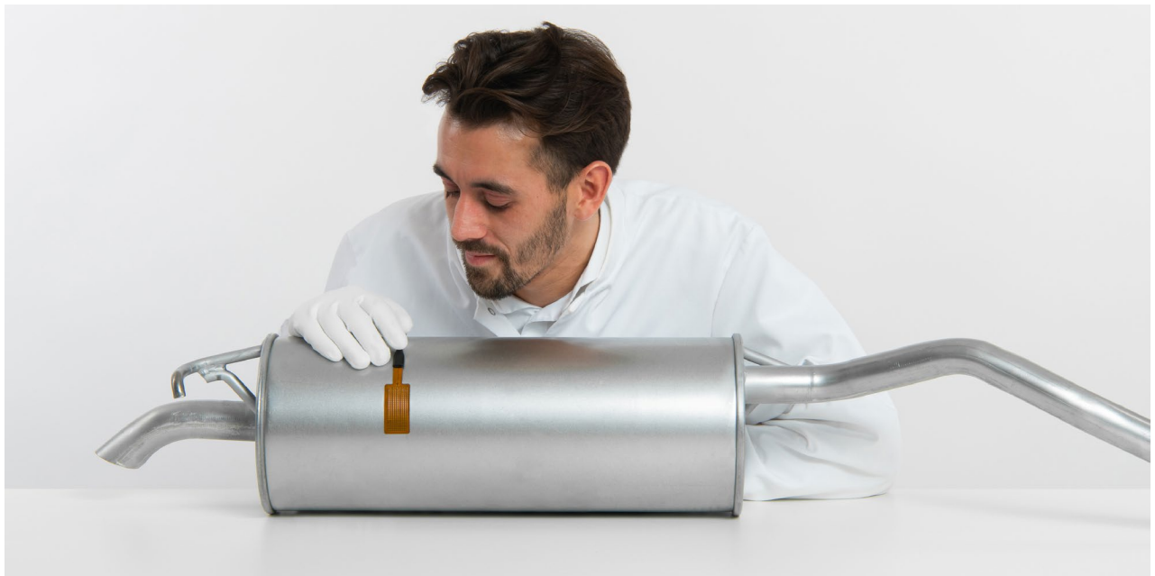
Figure 4.1.1 Example of model FHF06 high temperature foil heat flux sensor being installed for measurement on a car exhaust. FHF06 is flexible and can be easily mounted on a curved surface like a pipe or tube.
