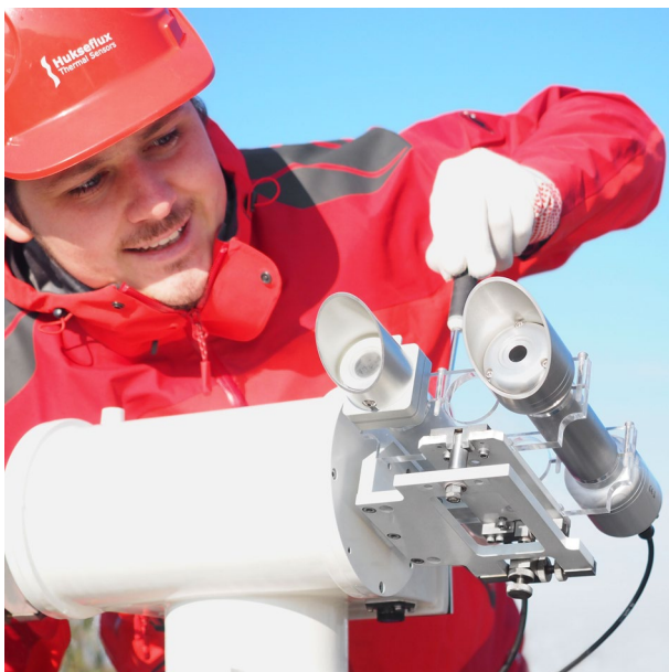
Figure 2 The importance of heating: tracker-mounted operation of DR30 pyrheliometer (on the right) compared to a non-heated instrument (on the left). The data availability of the non-heated instrument suffers in almost all environments due to morning dew, rime and frost.
