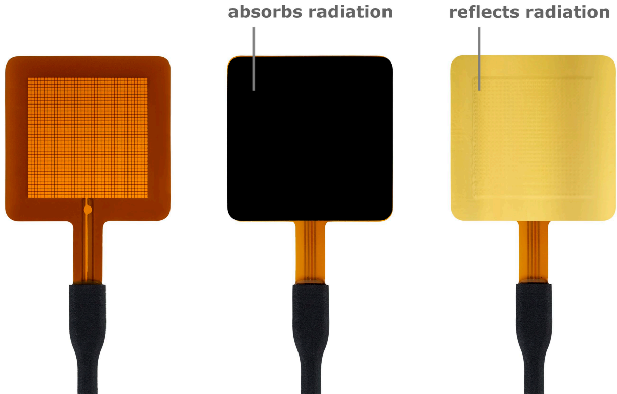
Figure 0.1 From left to right: model FHF05-50X50 heat flux sensor, FHF05-50X50 with BLK-50X50 sticker, and FHF05-50X50 with GLD-50X50 sticker. BLK – GLD stickers are also available for other dimensions of the FHF05 series and HFP01 heat flux sensors. The BLK black absorbing stickers will absorb all radiation and are sensitive to both radiative and convective heat flux, while the GLD gold reflective stickers reflect all radiation and are sensitive to convective heat flux only.
