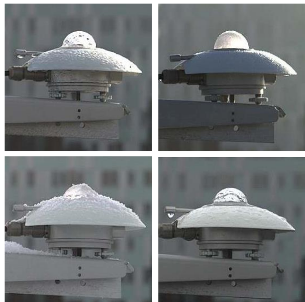
Figure 6 Dew (top left), frost (top right), snow (bottom left) and rain (bottom right) can affect pyranometer readings.
