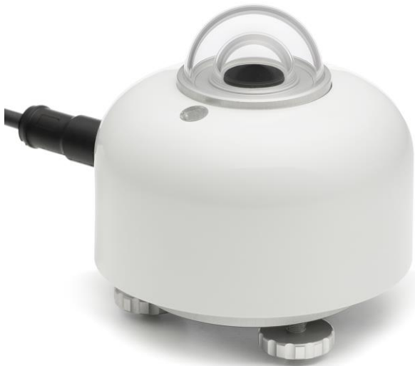
Figure 5 SR15 is a spectrally flat Class B pyranometer with two glass domes. The double dome construction provides better shielding against infrared thermal exchange than a single dome, reducing measurement offsets.
