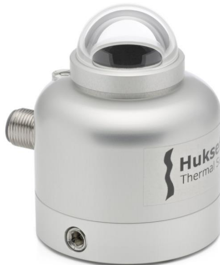
Figure 4 SR05 is a spectrally flat Class C pyranometer. It has a single glass dome to insulate the sensor surface from infrared thermal exchange with the colder sky. In addition, the dome protects the sensor against the elements.
