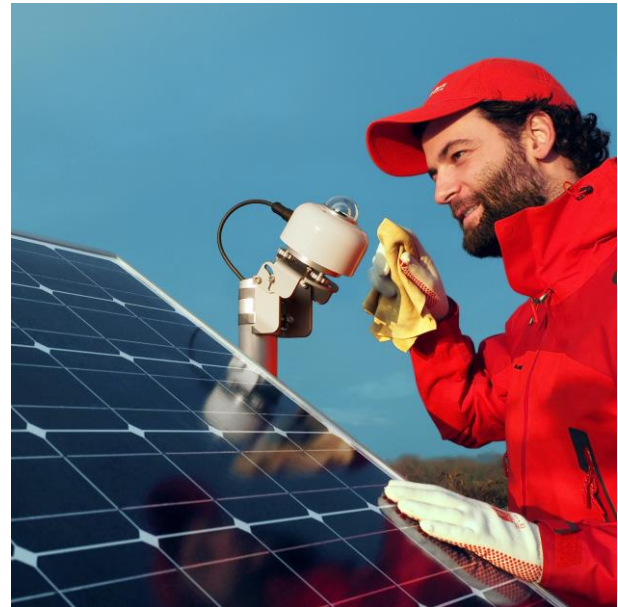
Figure 2 pyranometers can be used to monitor the performance of photovoltaic systems
