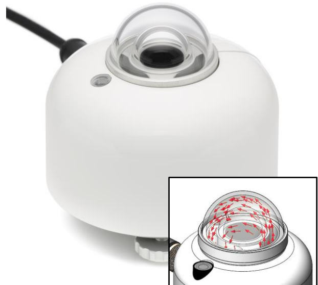
Figure 6 SR30 is a spectrally flat Class A pyranometer with two glass domes. Recirculated heated air through the sensor body and between the inner and outer domes creates a uniform temperature distribution throughout the sensor, resulting in a negligible infrared thermal exchange.
