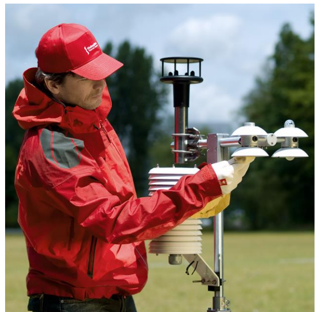
Figure 2 NR01, including a downfacing pyranometer, installed on meteorological station. The boom on which the NR01 is mounted should extend towards the equator
