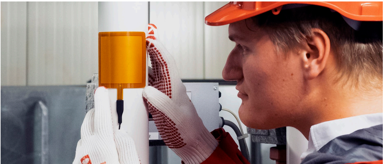
Figure 1 Model FHF05-85X5 heat flux sensor on a pipe to study heat losses.
