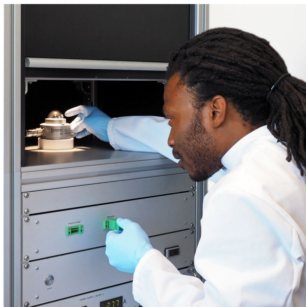
Figure 2 Application example: sensor being prepared for calibration in an indoor calibration system
