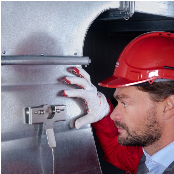
Figure 2 Verification of thermal behaviour of industrial equipment with the very robust IHF02 sensor. Here on a frame with magnets for surveying.
