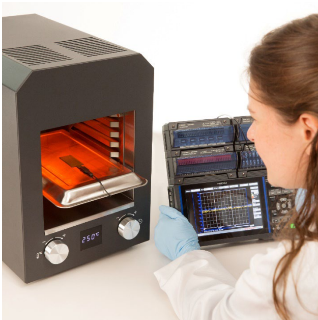
Figure 1 High temperature foil heat flux sensor model FHF06-25X50 used with Hioki LR8450-01.
