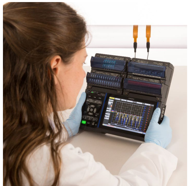
Figure 3 Hioki LR8450-01 can display voltage and temperature data of multiple sensors simultaneously on screen.
