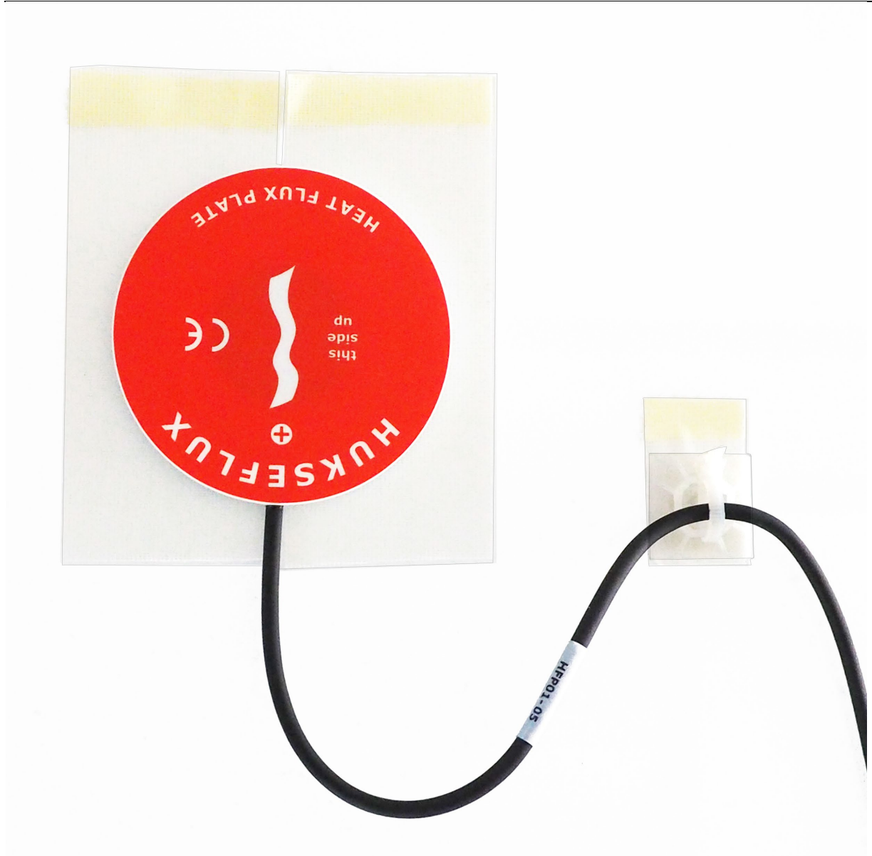
Figure 6.1.1 Installation of HFP01 on a wall using two-sided "removable" floor laying tape such as TESA 4939, and a strain relief of the cable using a cable tie mount equipped with the same floor laying tape as adhesive. TC temperature sensors may be mounted in the same way.
