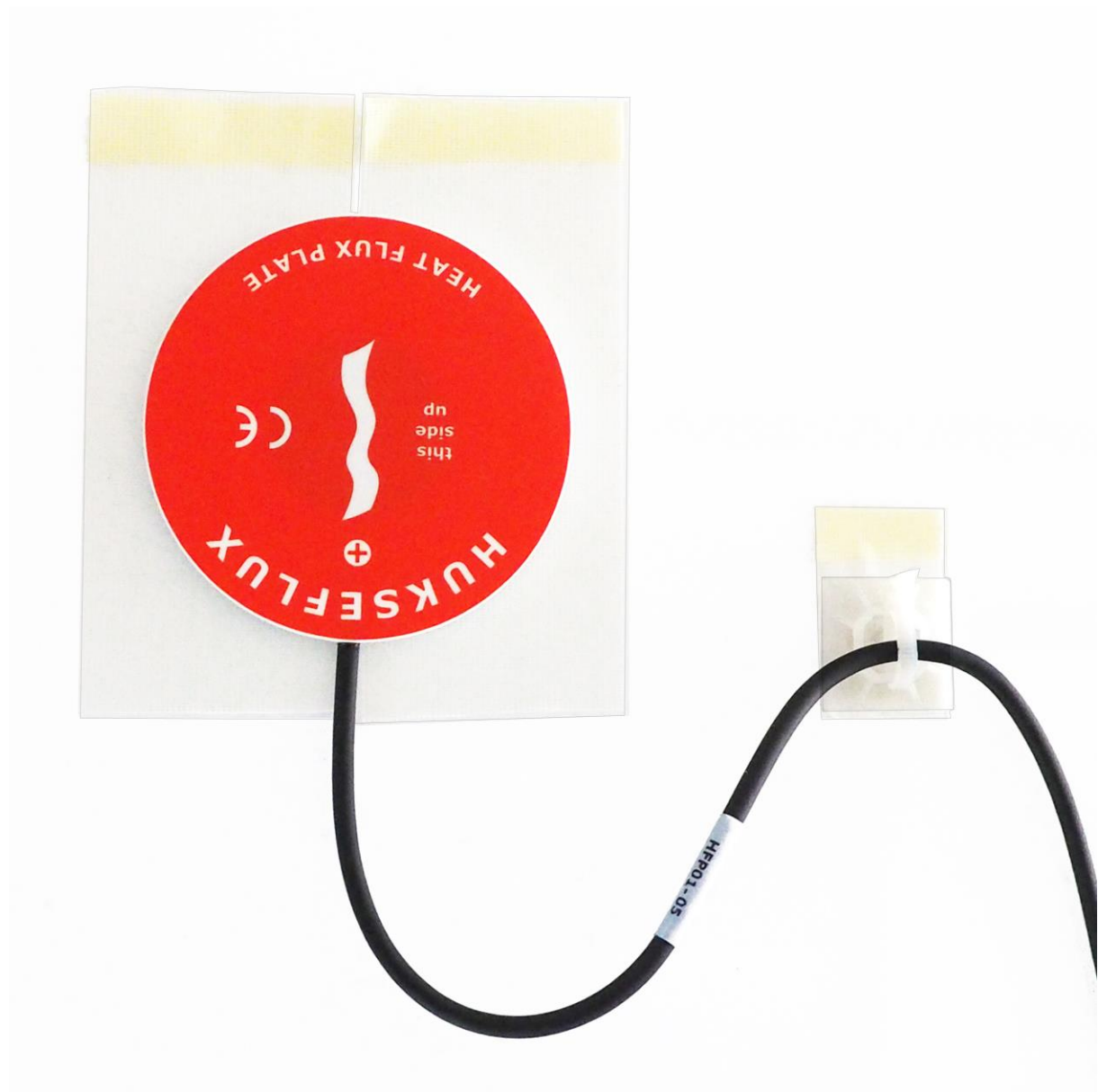
Figure 7.1.1 Installation of HFP01 on a wall using two-sided "removable" carpet laying tape such as TESA 4939, and a strain relief of the cable using a cable tie mount equipped with the same carpet laying tape as adhesive. TC temperature sensors may be mounted in the same way.
