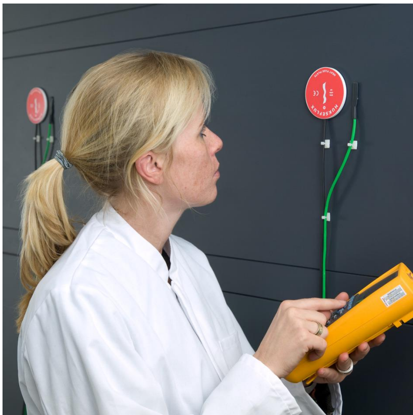
Figure 4.1 HFP01 heat flux sensor and TC mounted on a wall
