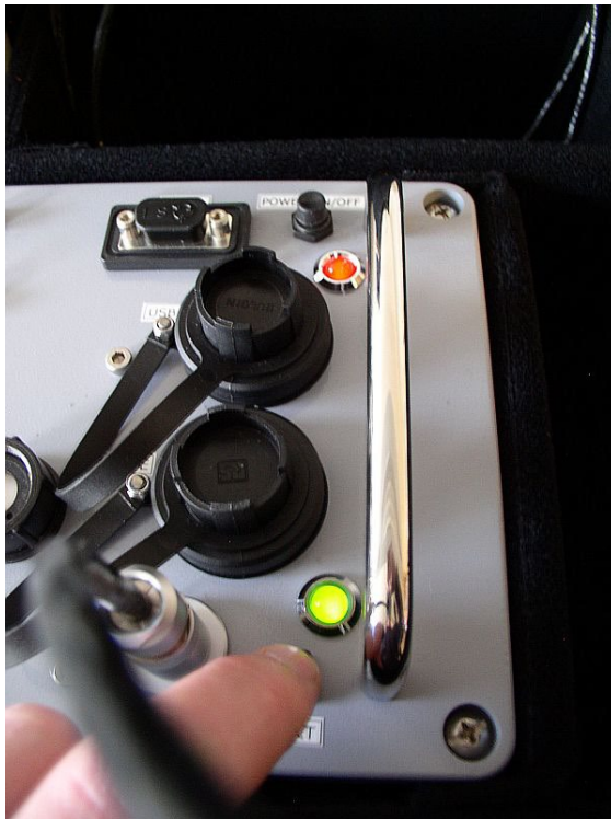
Figure 8.12.3 Arctic System special features: 1 above: power switch: Red: on 2 below: measurement switch. Green flashing: on, green burning: heating 3 in between: connectors for USB and charging
