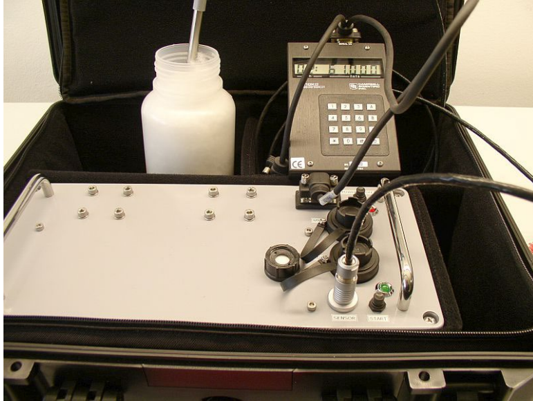
Figure 8.12.2 Arctic system measuring in glycerol, with keyboard display
