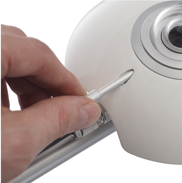
Figure 5.2.1 Installation and removal of SRA20's sun screen
