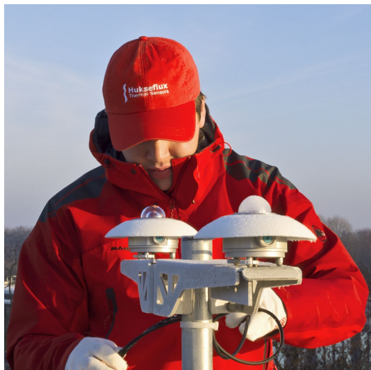
Figure 8.1.1.1 Heating of SR25 improves data availability; it keeps the outer dome free of dew- and frost deposition. This figure shows a heated SR25 (left) and an unheated pyranometer without sapphire dome (right) on a frosty morning.
