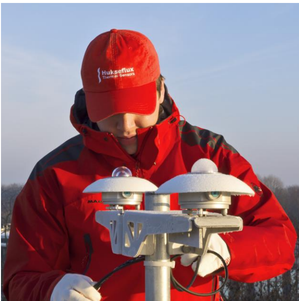
Figure 2 extensive testing of sensors, here outdoors on a frosty morning: clear difference between SR25 (left), versus an unheated pyranometer without sapphire dome (right)
