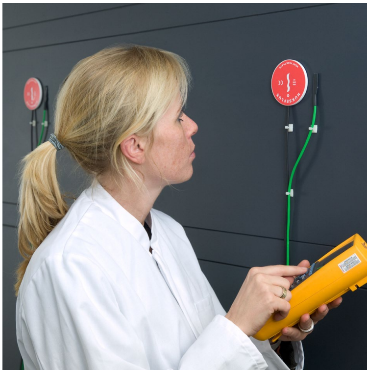
Figure 4.1.1 HFP01 heat flux sensors in use on a wall
