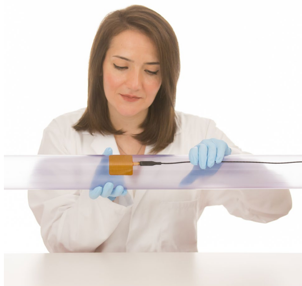
Figure 0.2 Application example: FHF05SC-50X50 being installed to measure heat flux on a pipe. The sensor is mounted on a well-prepared curved surface.
