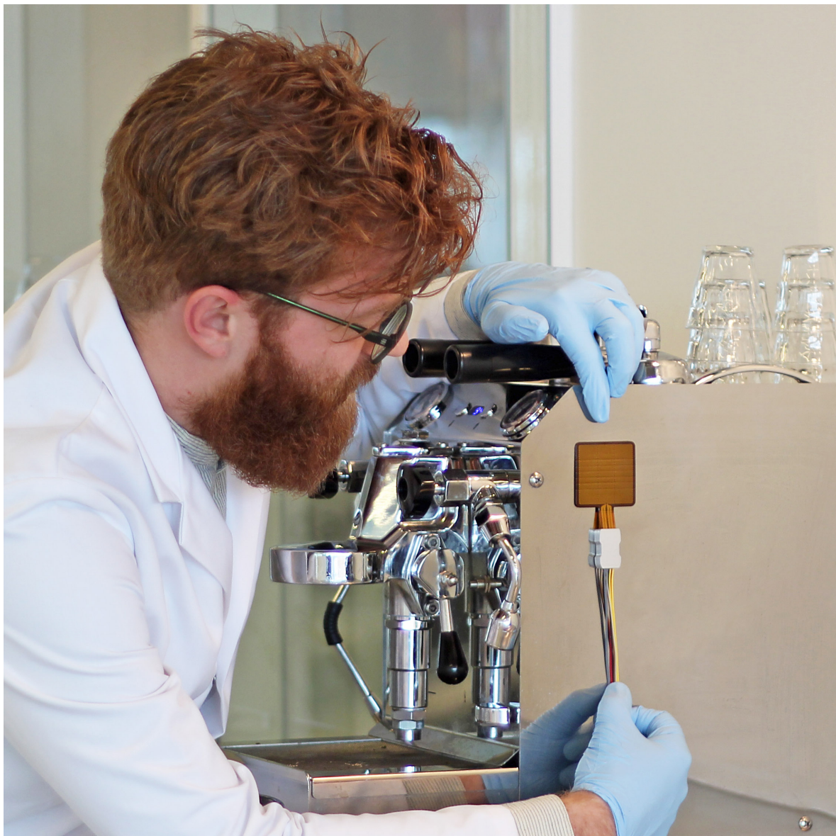
Figure 4.1.1 Example of a foil heat flux sensor being installed on an object. The sensor is mounted on a well prepared flat surface. Wiring must be provided with strain relief.
