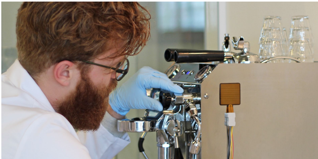
Figure 0.2 An application of FHF02SC self-calibrating foil heat flux sensor
