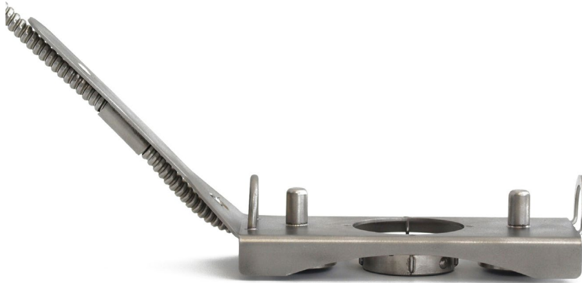
Figure 0.2. HF01 heat flux and surface temperature sensor with frame with magnets
