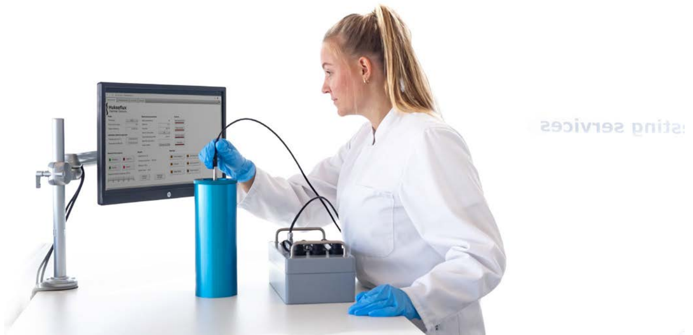
Figure 0.1 Application of the complete TPSYS20 measuring system in a laboratory environment using a CRC01 calibration reference cylinder
