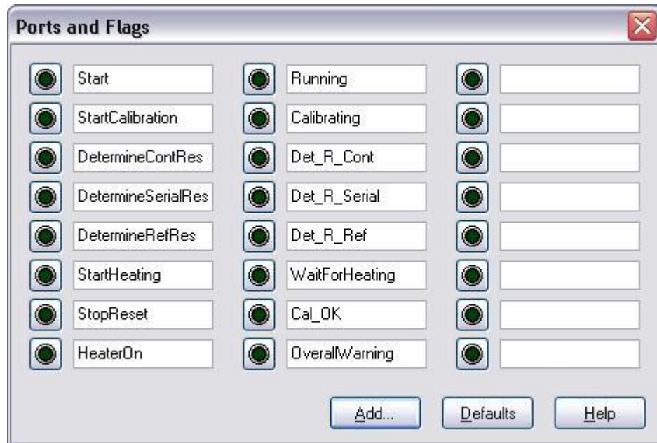
Figure 5.5.3 The control screen after variables have been added. The buttons can be pressed to activate programmed procedures and to read of the status of the MCU.
