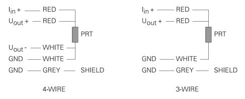
Figure 8.1 *ST01* in a 4-wire connection (preferred) or a 3-wire connection.
