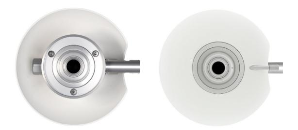
Figure 0.2 SRA20 secondary standard albedometer, seen from below and from above
