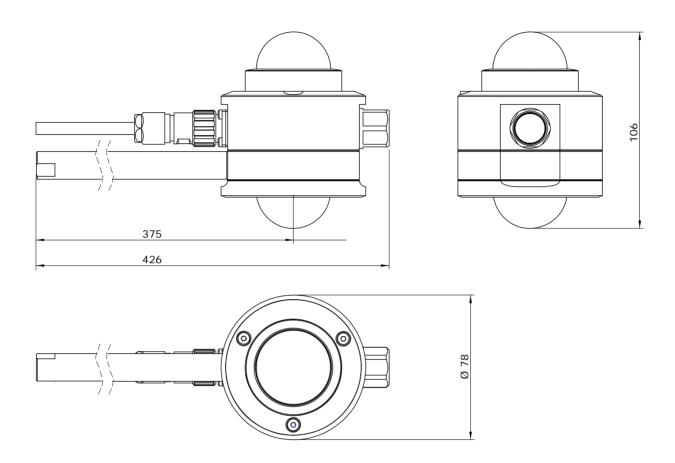
**Figure 3.3.1** Dimensions of SRA20 in  $10^{-3}$  m. The mounting rod has a 15 x  $10^{-3}$  m diameter
