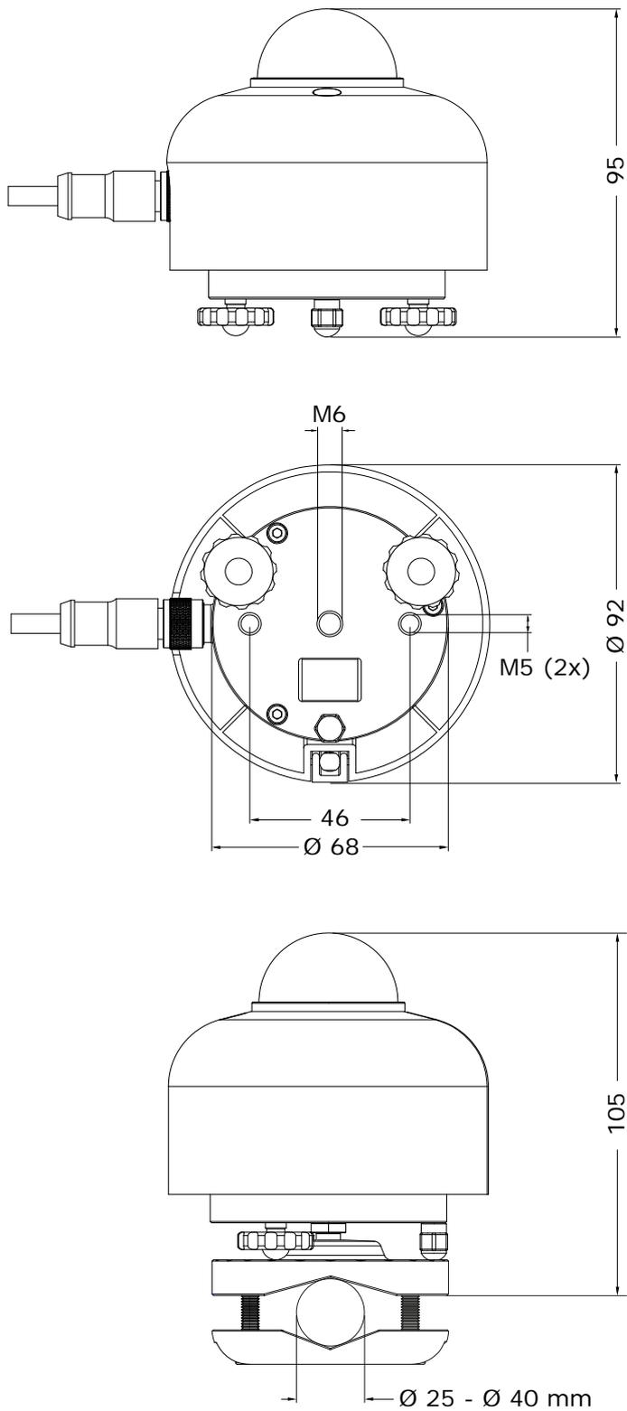
**Figure 3.2.1** Dimensions of SR30 in  $\times 10^{-3}$  m. Mounts are optional
