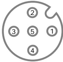
**Figure 6.5.1:** *Connector layout of SR30, indicating PIN numbers (viewed from cable side)*
