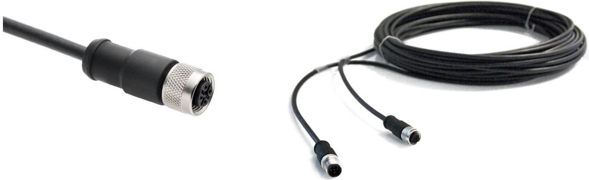
**Figure 0.7** *On the left the SR30 cable with M12-A female connector on sensor end, pigtails of 0.15 m and conductors with ferrules. Its length is 5 metres standard and available in 10 and 20 metres too. On the right the optional Hukseflux extension cable with connector pairs, with male and female M12-A connectors, available in 20 metres*
