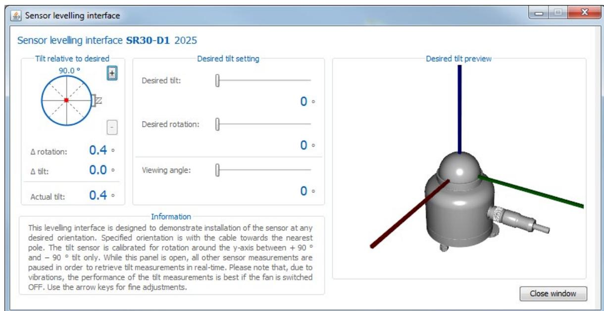
**Figure 7.1.8.1** Sensor levelling interface in the Sensor Manager
