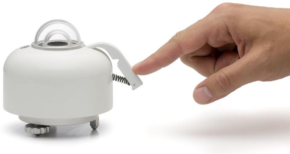
**Figure 6.2.2** *Installation of SR30's sun screen*
