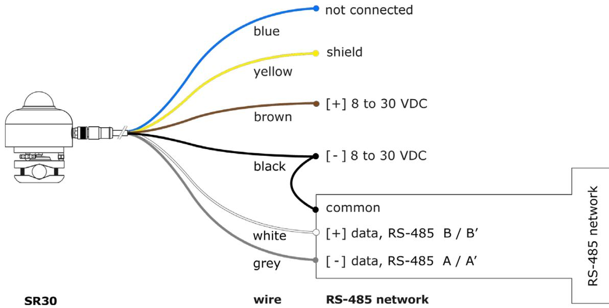
**Figure 6.7.2** Connection of SR30 to an RS-485 network. SR30 is powered by an external power supply of 8 to 30 VDC.
