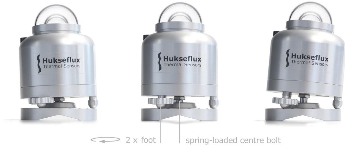
**Figure 6.3.1.5** SR30 locked on its optional levelling mount: by fastening (on the left) or loosening (on the right) SR30's two adjustable feet, SR30 can be levelled, judging by the bubble level. SR30's static foot remains fixed. In all cases, ensure the legs of SR30 fit into one of the small ledges of the levelling mount. Locking is in place, when the nut is turned all the way against the bottom plate of SR30
