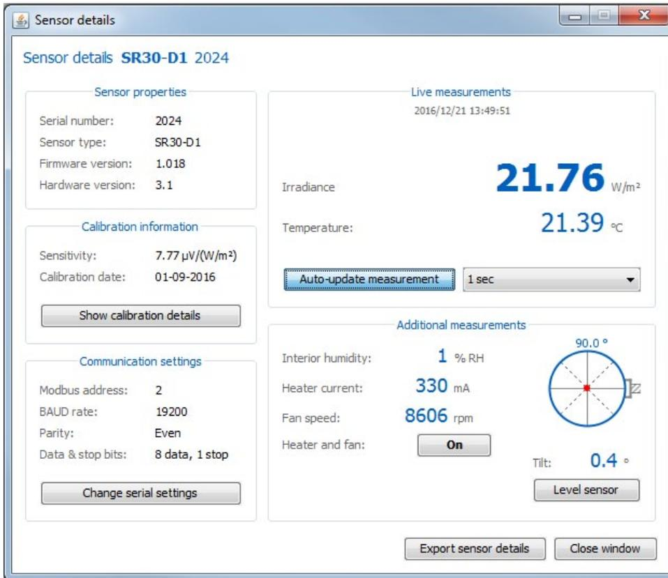
**Figure 7.1.5.1** *Sensor details window in the Sensor Manager*
