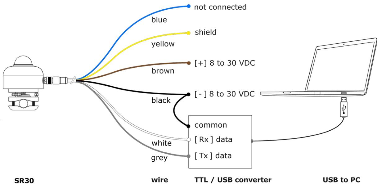
**Figure 6.8.1** Connecting SR30 to an RS-485 to USB converter and a PC
