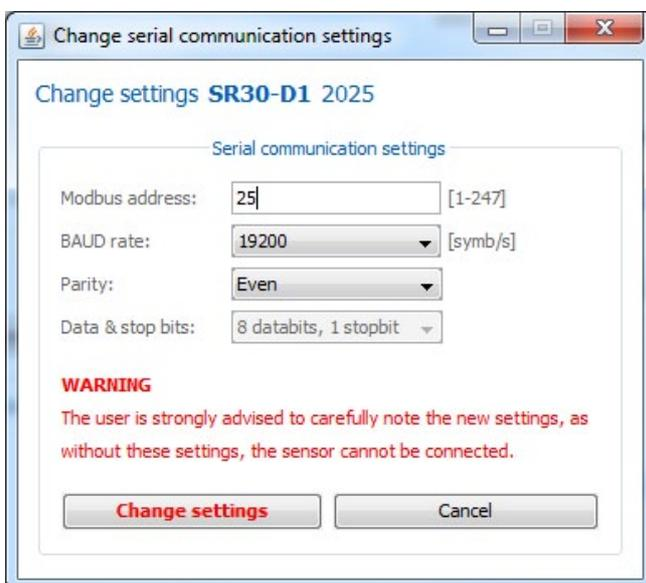
**Figure 7.1.6.1** *Change serial communication settings window in the Sensor Manager*
