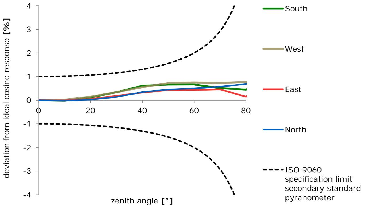
**Figure 2.0.3** Directional response of an SR30 pyranometer of 4 azimuth angles, compared to secondary standard limits.
