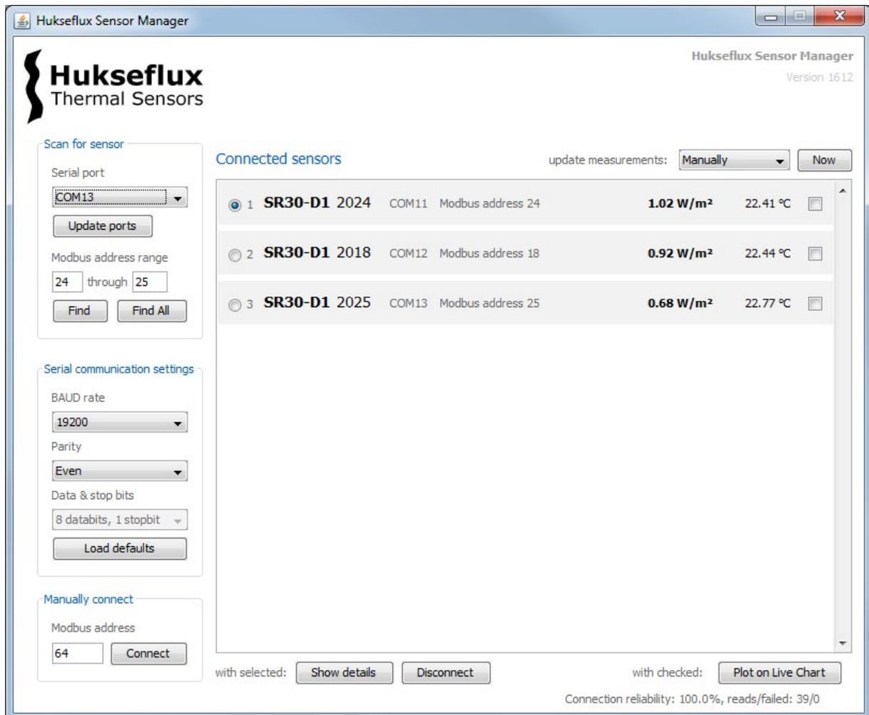
**Figure 7.1.3.2** Sensor Manager main window with three connected SR30's
