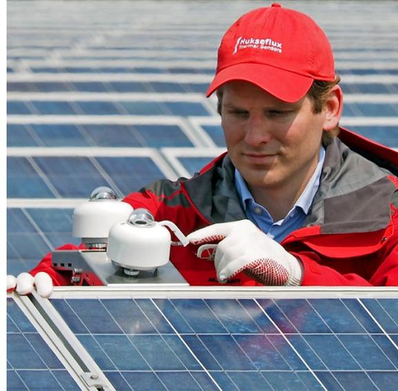
**Figure 0.3** Two SR30 secondary standard pyranometers with digital output for GHI (global horizontal irradiance) and POA (plane of array) measurement applications
