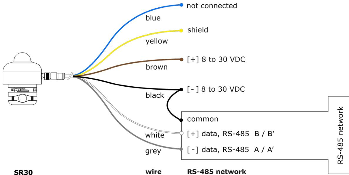
**Figure 7.3.1** Connecting SR30 to a typical RS-485 network
