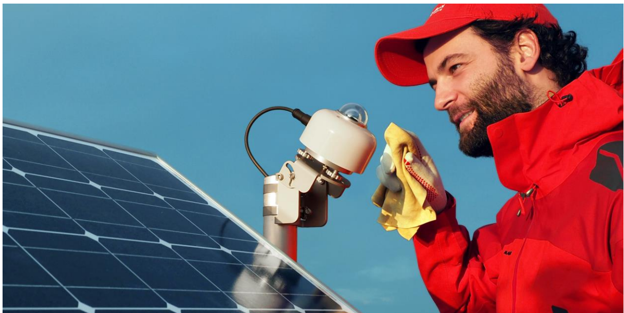
Figure 0.2 SR15 pyranometer mounted on a mast in PoA (Plane Of Array) for PV system performance monitoring
