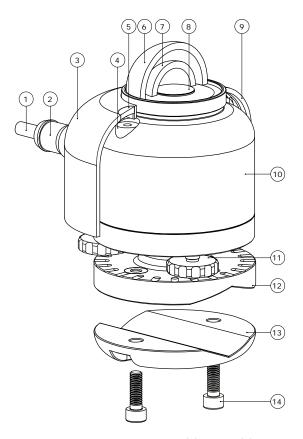
Figure 3 overview of SR15-A1: (1) cable, (2) connector, (3) sun screen, (4) bubble level, (5) bubble level window, (6) outer dome, (7) inner dome, (8) thermal sensor with black coating, (9) quick release system of sun screen, (10) instrument body, (11) levelling feet, (12) optional spring-loaded levelling mount, (13) optional tube mount, (14) screws included with tube mount
