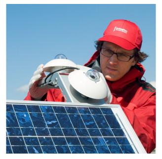
Figure 2 PV system performance monitoring pyranometers
