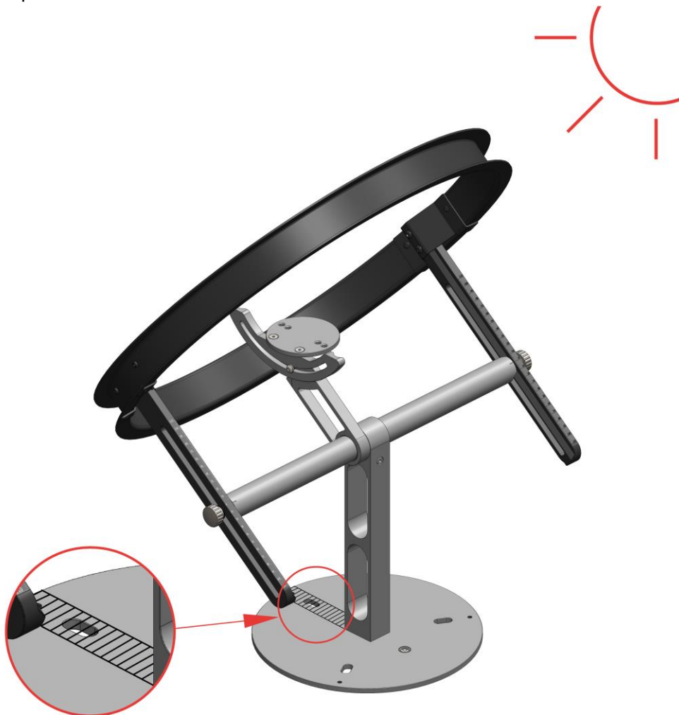
Figure 5.4.1.3.1 Aligning the shadow parallel to the vertical support
