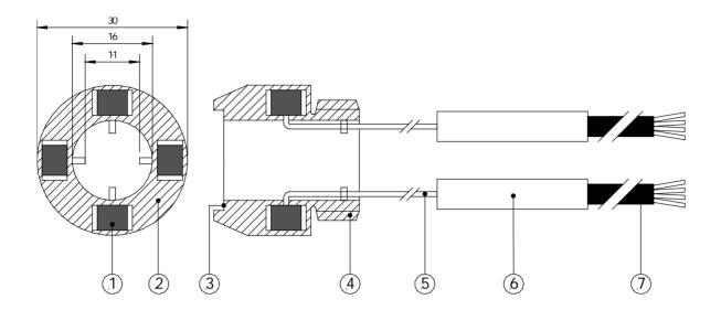
**Figure 2.1** Example of RHF01 ring heat flux sensor with 4 x heat flux / temperature sensors (1), in a stainless steel body (2), with either a flat connection for welding- (3) or a threaded connection (4). High temperature cable (5) is usually extended with low temperature extension cable (7). Cooling must be provided by air, oil or water. RHF design is user-specific. Dimensions in the drawing serve as an example only. Dimensions are in x  $10^{-3}$  m.
