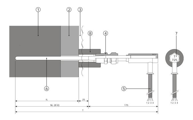
**Figure 3.2.1** NF01 standard version for operation in the furnace lining (graphite or brick) part of the furnace wall: (2) steel shell, (3) water, (1) graphite, (8) shell coupling, (4) screwed coupling, (5) cable, (6) needle type heat flux and temperature sensor.
