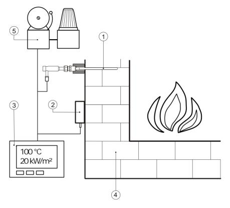
**Figure 0.5** Monitoring of furnaces and ovens: (1) needle type heat flux & temperature sensor NF01, (2) surface heat flux & temperature sensor model HF01 (not discussed in this document), (3) readout unit, (4) brick, (5) alarm/warning system
