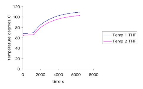
**Figure 7.2.1** Example 1: simulation of furnace overheating. Normal operation of the furnace until about 1000 s. Form then on the furnace starts overheating. In case of furnace overheating all temperatures as well as the heat flux rise. In this case the heat flux is increased by a factor 1.8.
