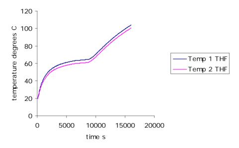
Figure 7.2.2 Example 2: simulation of cooling malfunction. Around 8000 s after initial start-up of the furnace, the water cooling is stopped. The temperatures rise quickly but the heat flux, after a temporary dip caused by thermal loading, stays close to normal. It will eventually stabilise close to the original heat flux at a higher absolute temperature. Please note that the heat flux signal has been corrected for the temperature dependence of the thermal conductivity.
