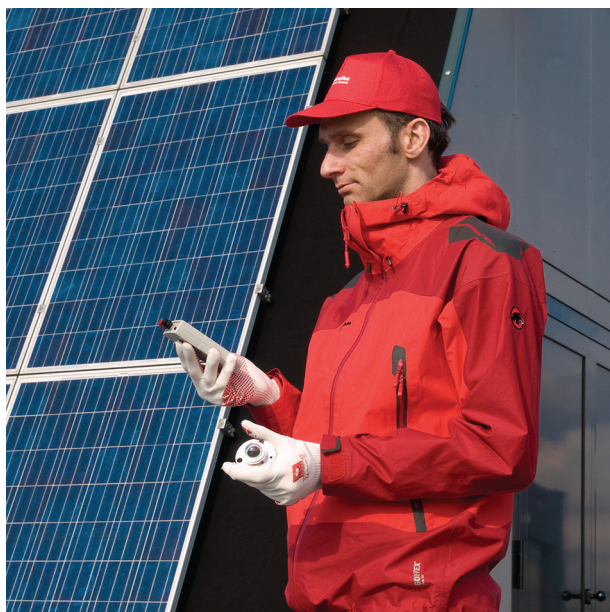
Figure 4 LI19 with a pyranometer in a field measurement
