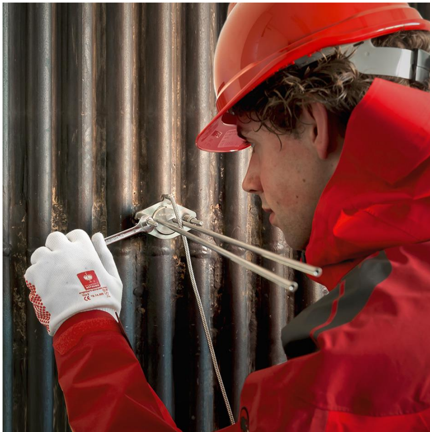
Figure 4.1.1 Industrial heat flux sensor mounted on a boiler wall using tack-welded threads and spring-loaded bolts. The sensor is mounted on a well prepared flat surface. Cabling must be provided with strain relief.
