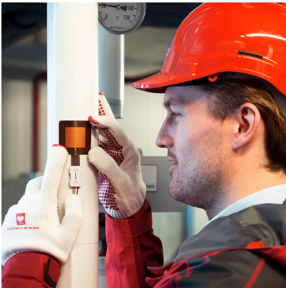
Figure 4.1.1 Example of an FHF04 foil heat flux sensor being installed for measurement on an industrial pipe. The sensor is mounted on a well-prepared curved surface.
