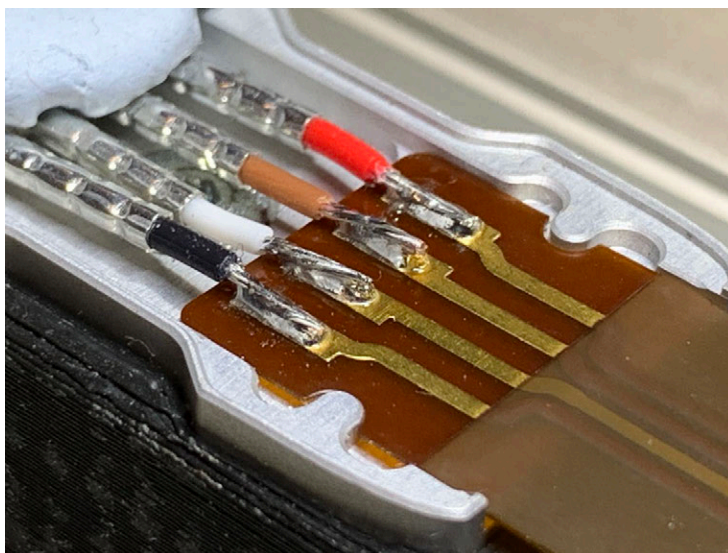
Figure 7.2.2 FHF04 sensor foil with soldered wires.
