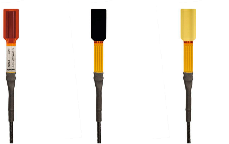
Figure 0.3 FHF03: with BLK-3015 and GLD-3015 stickers to measure radiative and convective heat fluxes separately
