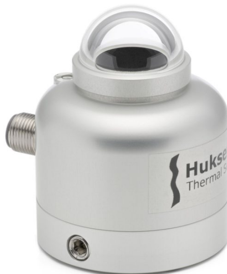
Figure 4 SR05 is a second class pyranometer. It has a single glass dome to insulate the sensor surface from infrared thermal exchange with the colder sky. In addition, the dome protects the sensor against the elements.
