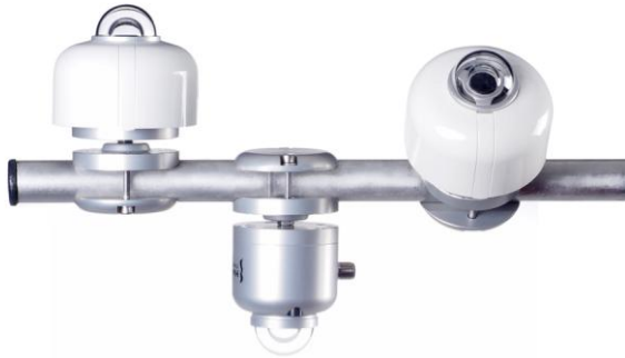
Figure 1 in PV system performance monitoring users typically employ Plane of Array (POA) Global Horizontal Irradiance (GHI) and increasingly also Reflected Irradiance (RI)
