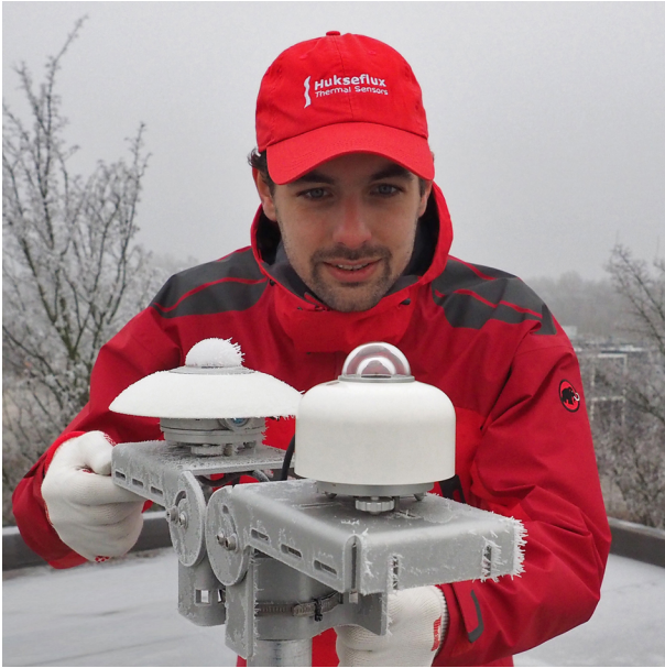
Figure 2 Hukseflux model SR30 is the first heated pyranometer, compliant with the requirements of IEC 61724-1 for Class A monitoring systems. It overcomes a typical problem in freezing conditions: ice accumulation on the pyranometer dome surface reduces data availability. At the front a new design with recirculating ventilation.
