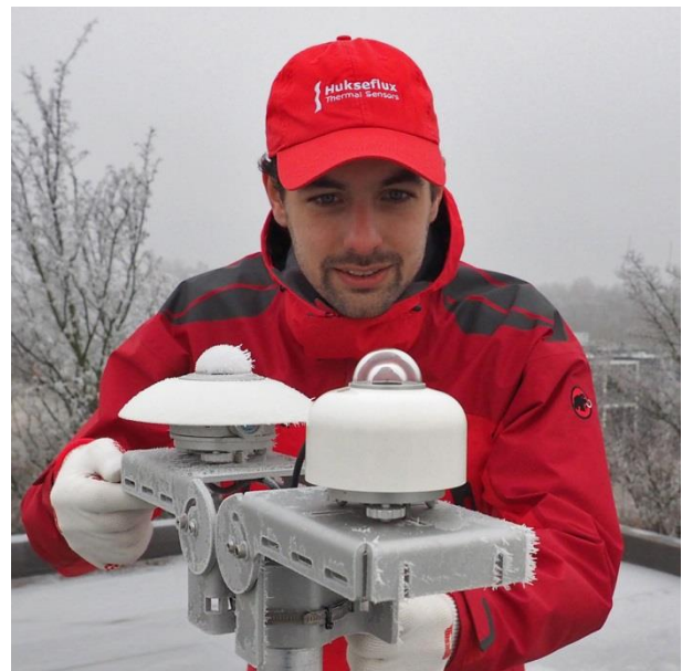
Figure 5 Frost and dew deposition: clear difference between a non-heated pyranometer (back) and the heated SR30.
