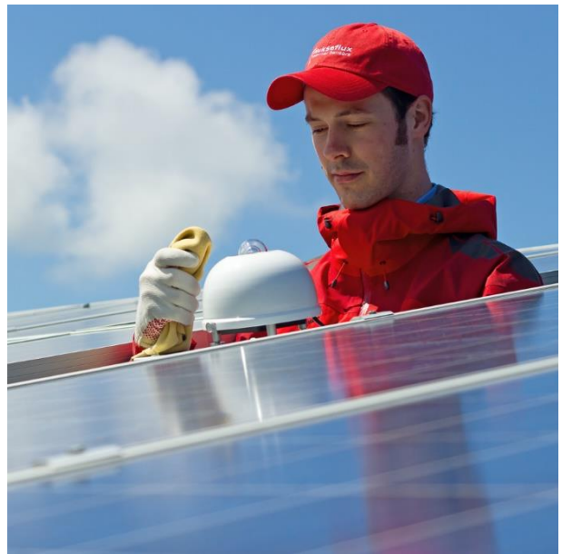
Figure 3 example of an externally ventilated pyranometer, here in use for PV system performance monitoring
